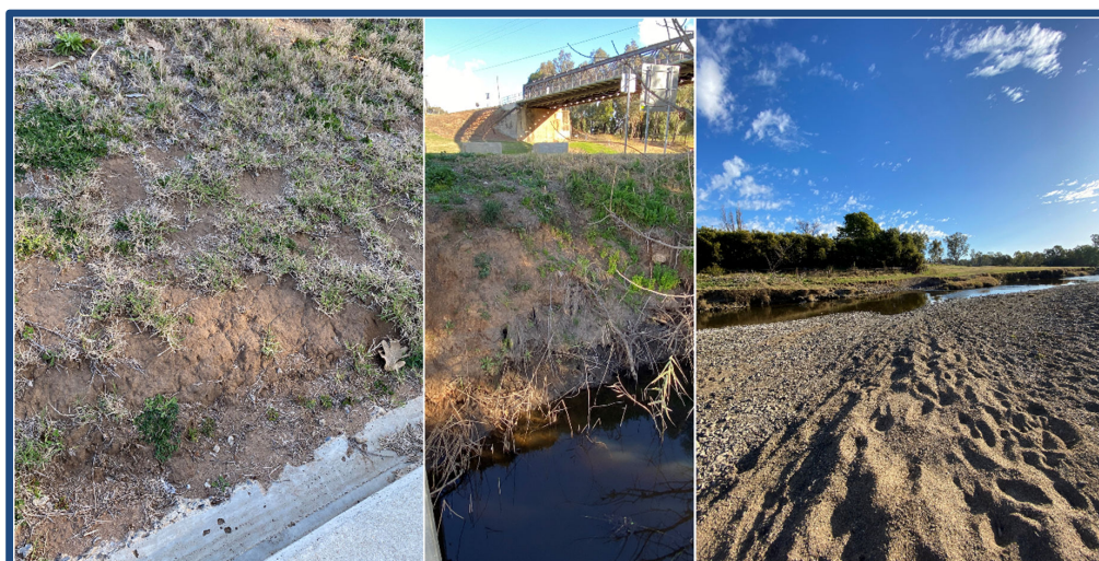
Figure 9 – Soils at the Gwydir Riverside Bingara (Left to right): Silty clay loam ( Tenosol ) of the elevated flood levee; Silty soil of the riverbank levee ( Tenosol ); Sands and gravels above the junction of Halls Creek and Gwydir River ( Rudosols ).
