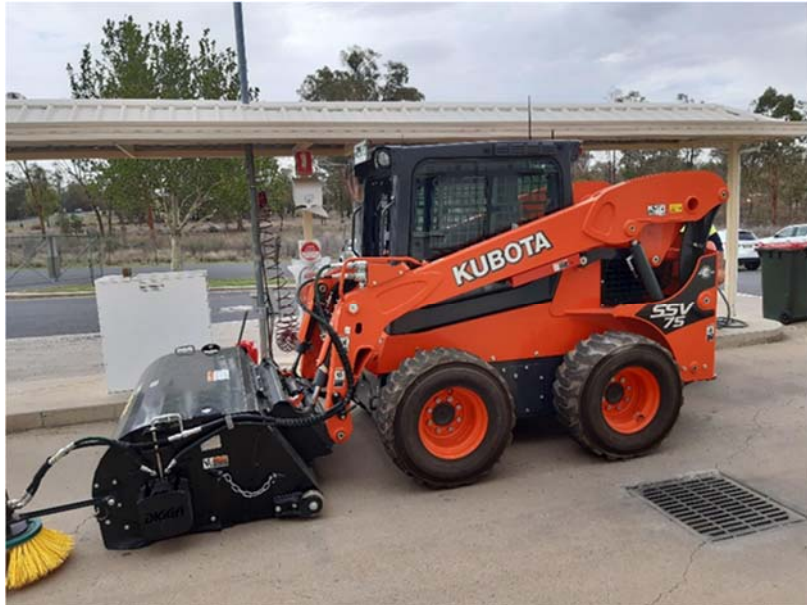
New skid street loader street sweeper
