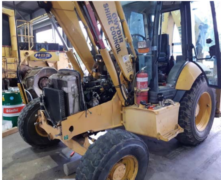
P1625 Komatsu backhoe in the workshop to have a cylinder heads gasket replaced
