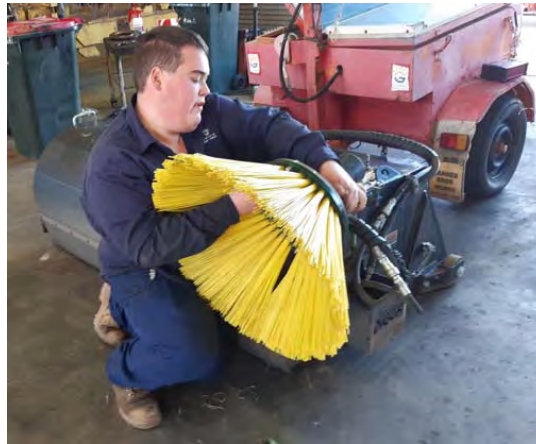
Bray Logan replacing brushes on P1950 skid steer sweeper
