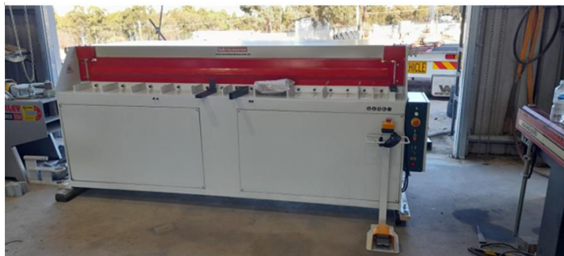
Guillotine for use in fabrication workshop
