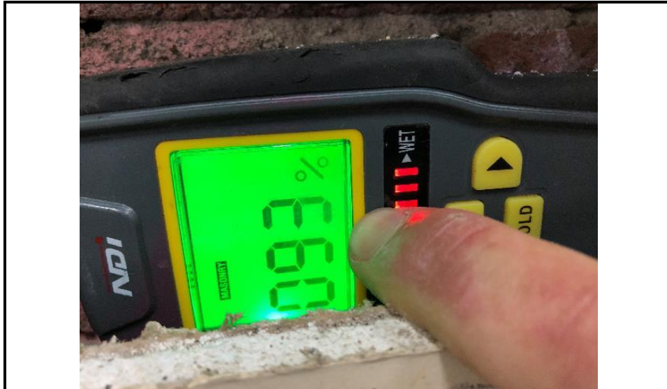
Photograph 39: Shows the moisture level to the existing external brick walls behind the office fit out.
