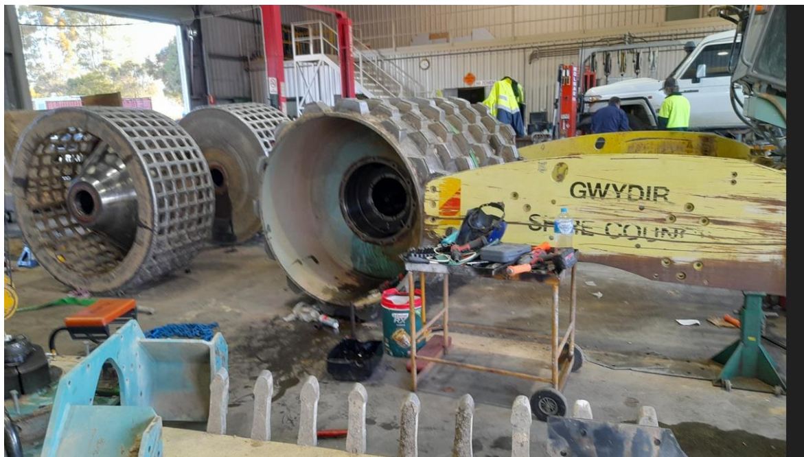
P1474 – pad foot roller - bearing replacement
