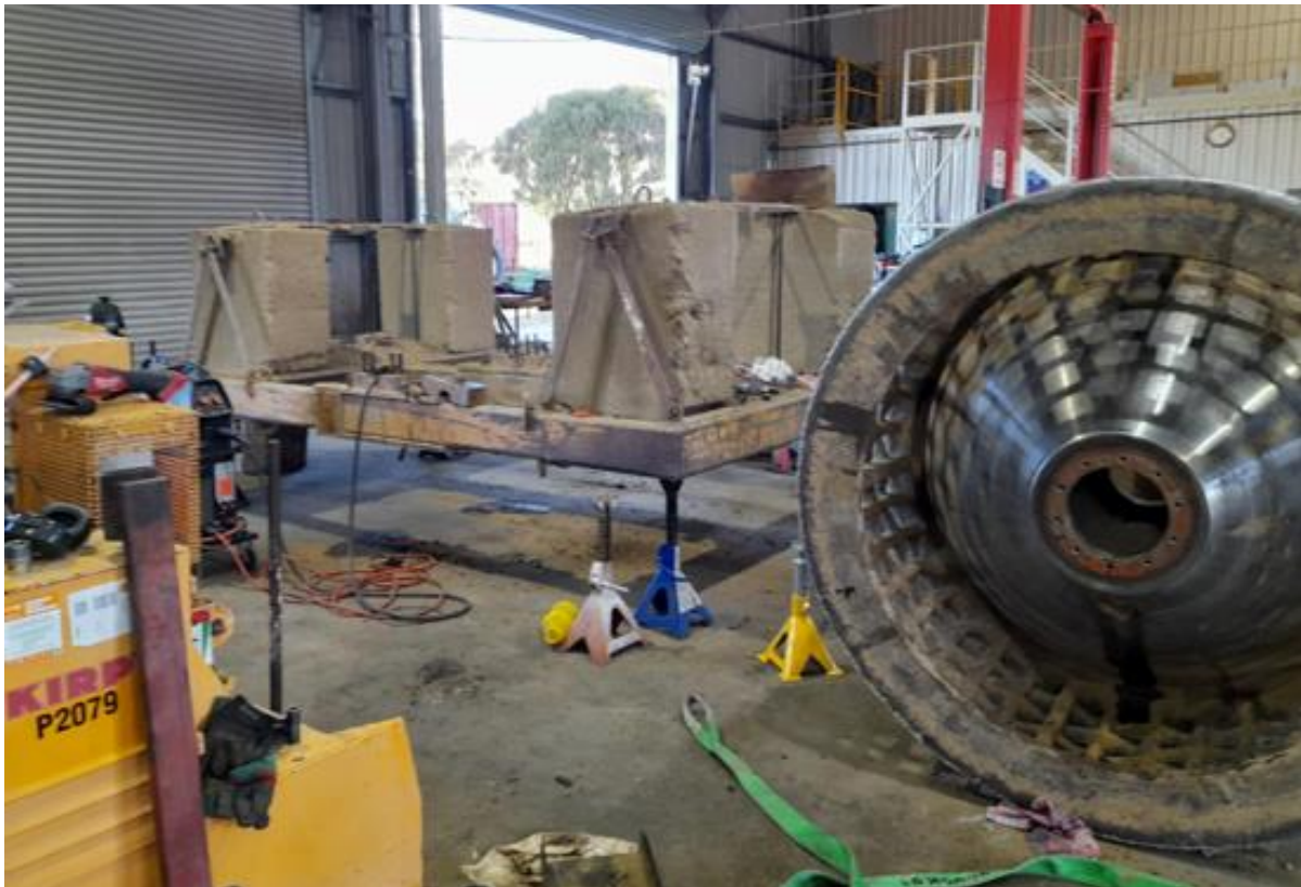
P1134 Grid roller from Bingara had bearings and seals replaced Warialda workshop
