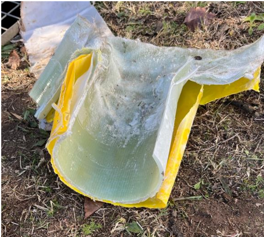
Sample of pipe relining
